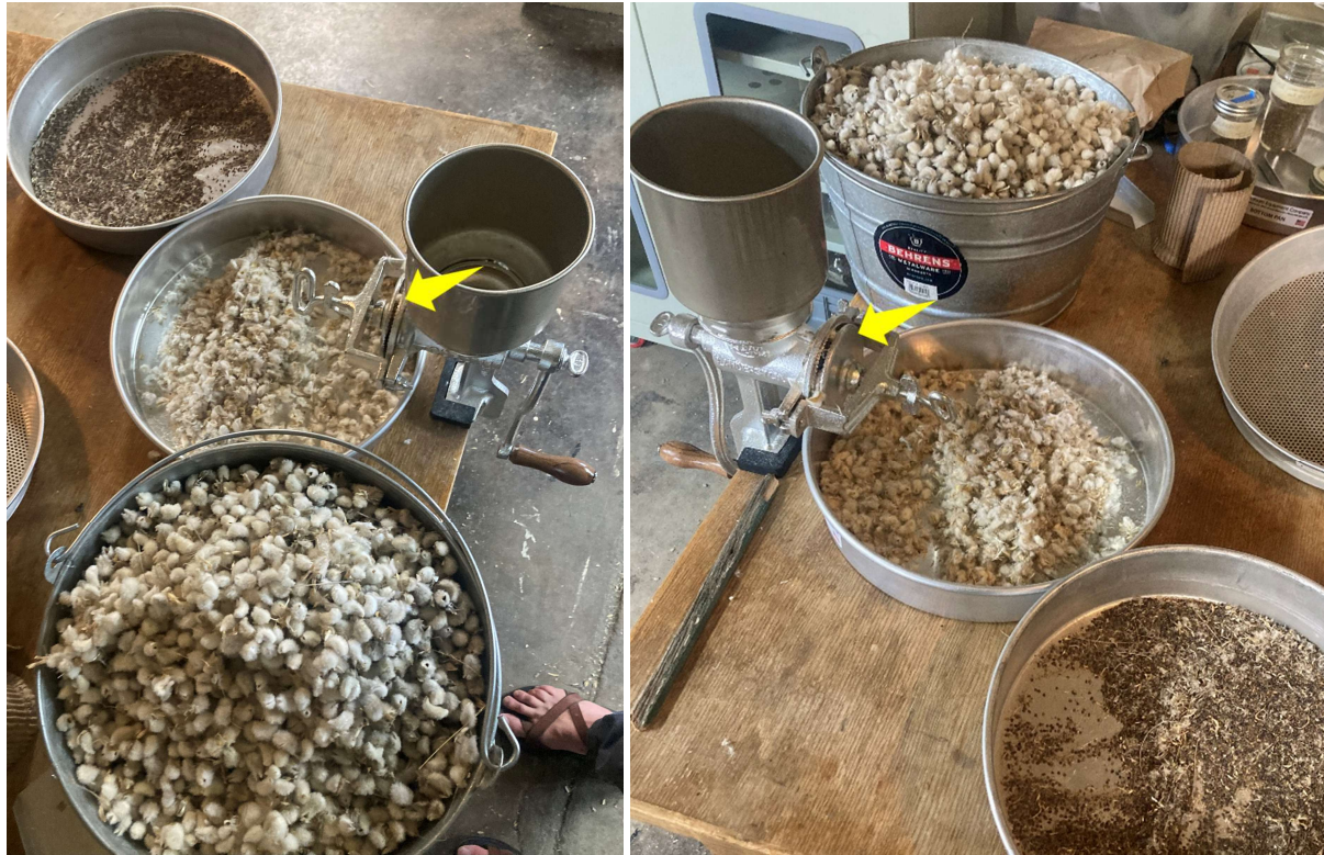
Figure 10. The acquisition of a $40 grain mill allowed for efficient and more complete extraction of woolly milkvetch seeds from their durable, sharp, velvety pods. By adjusting the gap of the grinding plates to the correct width (yellow arrows), the whole pods (bottom left) were easily broken open enough for seed to readily be sifted out (bottom right). This process saved hours over prior methods of processing in small batches in the barrel chain thrasher, followed by hand-peeling of pods that refused to open. We used our air separator on the extracted seed to assess seed damage, and confirmed it was very low.
