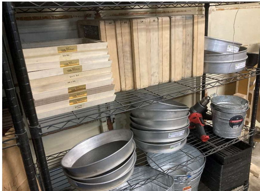
Figure 11. The current set of sieves used by the Program, including various sizes of three different styles: fine wire mesh (top left), coarse wire mesh (top right), and perforated metal pans (bottom).
