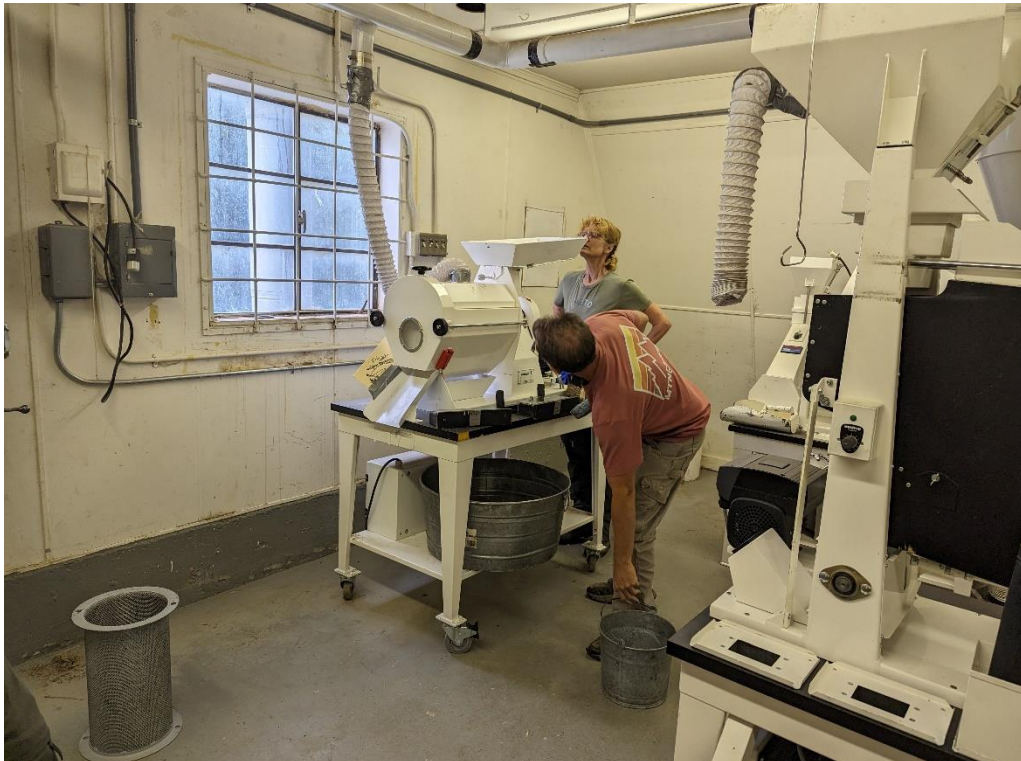
Derek Tilley demonstrating the use of the LA-H Laboratory Brush Machine to Diane.
