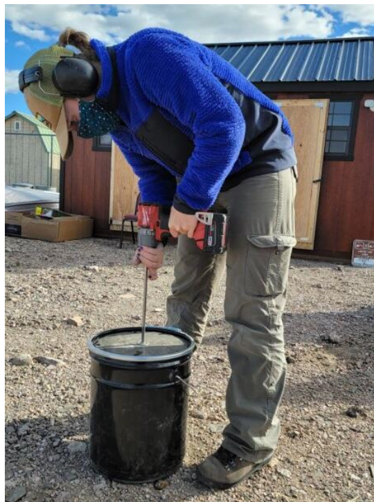
Katie Baumann using our 5-gal DIY drum thresher to break open Astragalus seed pods.
